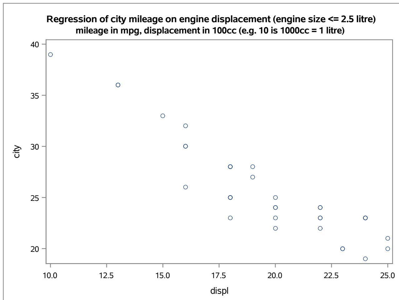
**Regression of city mileage on engine displacement (engine size <= 2.5 litre)**
