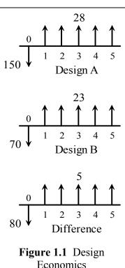
Both designs solve the problem. Design A is more technically advanced, but design B is adequate. Examine the differences in the cash flows of the designs, shown at the bottom of Figure 1.1. The technical advances of design A provide extra savings of \$5,000 per year for five years, but these savings cost \$80,000 more initially. The extra benefits clearly are not worth the extra costs. The objective of a company is to make money, so the graduate producing design B is the more valuable employee.
